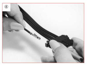
\* Insert the jig top into the peak of convex section on terminal hole.
